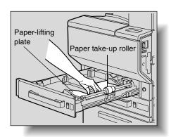
3 Slide the lateral guides to fit the size of paper to be loaded.
